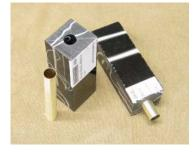
II. To glue in the tubes use a medium CA adhesive and wear gloves. This should be done in a well-ventilated area to avoid the CA fumes. First apply a small amount of CA to the inside of the first blank hole at the matched end. Run it around the entire hole circumference. Stand the blank on end so the CA runs down through the hole.
