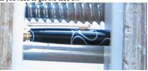
6. Finally, slip the centre band over the twist mechanism, and then push the upper barrel on with a twisting motion. Your pen is now complete.
