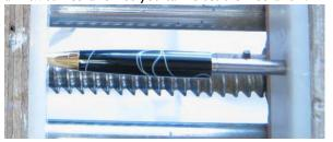
4. Remove from the press and insert the refill. Ensure it extends enough for comfortable writing. If not, press the twist mechanism in a little further and re-check.
