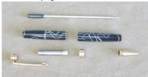
2. Using a press or bench vice, press the writing tip into the lower barrel. Take care to ensure the tip is correctly aligned before pressing it in.
