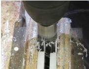
17. Once milled, remove any burrs on the inside of the brass tube. This will also aid with assembly of the finished pen.
