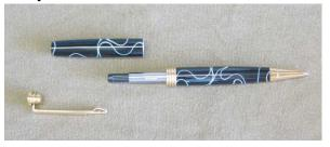
5. Next, slip the clip over the cap then press the cap into the upper barrel. The clip can at times be quite tight on the cap, it may be necessary to press it on using a suitable piece of tube. Note: don't use a brass pen tube as you need to get the tube off.
