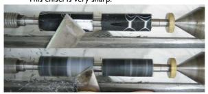
During roughing the Acrylic will tend to come off in pieces. Care should be taken when cutting towards the blanks end as the Acrylic can chip away if excessive force is applied to the chisel.
