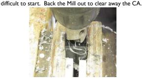
16. Next, using gentle downward pressure, start to mill the end of the pen. Take care and take your time, excessive pressure can heat the Acrylic up and cause it to soften. Mill the blank until the brass tube is reached. Back the mill away from the blank as you mill to check progress. Repeat this for each end of the two blanks.
