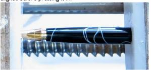
3. Then press the twist mechanism into the lower barrel. Be careful not to push this in to far. Again, ensure the twist mechanism is correctly aligned before pressing. If you do push it in to far, the 7mm Pen Disassembly Tool can be used to remove the writing tip and twist mechanism so you can re-set the mechanism.
