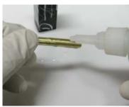
13. Insert the brass tube into the blank from the matched end. Work it in and out a couple of times while turning it to ensure a good even coverage of CA inside the blank. Then push the tube in to approximately I-I.5mm under flush with the matched end.
