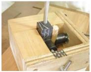
7. Carefully drill out the blank using a 7mm drill bit. Make small advances with the drill, backing it out often and allowing the shavings to clear out of the drill flutes. Take care near the end of the drilling; excessive pressure on the drill may cause the acrylic to chip away from the hole edges as the drill exits the blank.
