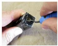
18. The blanks are now ready to mount on the mandrel in the lathe.
