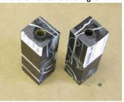
15. Once cured, hold each blank in a vice or similar. Using a battery drill on high speed carefully run the Pen Mill into the brass tube to clear out any CA. If there is CA build-up in the end of the tube the mill can be
