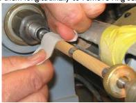
2. Use a soft foam block to help finish the shaping of the pen if required.
