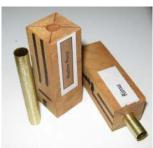
10. To glue in the tubes use a medium CA adhesive and wear gloves. This should be done in a well-ventilated area to avoid the CA fumes. First apply a small amount of CA to the inside of the first blank hole at the matched end. Run it around the entire hole circumference. Stand the blank on end so the CA runs down through the hole.
