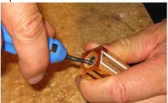
17. The blanks are now ready to mount on the mandrel in the lathe.
