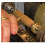
A good method for doing this is to turn a shallow taper at the end of each blank, always working toward the blank end.
