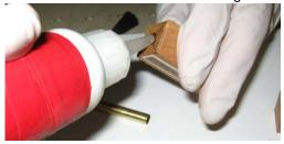
II. Apply CA to the brass tube in beads around the tube. Rotate the tube in your fingers to get a fairly even spread.
