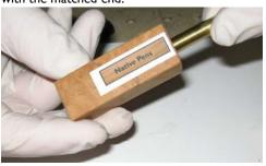
13. Check to ensure that both ends of the blank have glue coverage around the tube ends. If it looks a little dry you can wipe a bit of CA around the tube at the end with you finger and allow it to wick back along the blank inside. Allow the CA to cure overnight.
