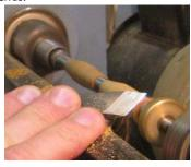
Once again turn the tapers on the blank ends, leaving the end diameter of the blank about 1-0.5mm larger than the bushing.
