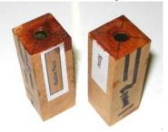
I4. Once cured, hold each blank in a vice or similar. Using a battery drill on high speed carefully run the Pen Mill into the brass tube to clear out any CA. If there is CA build-up in the end of the tube the mill can be difficult to start. Back the Mill out to clear away the CA.
