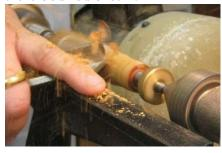
Stop the lathe and check the blanks for any defects exposed in this stage. If there is a defect you can decide to keep it and continue as it might be turned off before the pen is finished or to turn the wood off the tubes then start again. Remember, a small defect can be hidden behind the clip during assembly.
