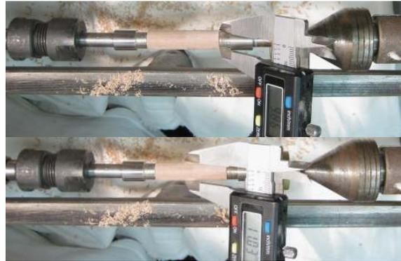
4. Sand down the Mill Bush until it is very close to the lower part of the bushings.
